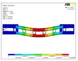
Fig 8: Natural Frequency mode – 1 Deformation
