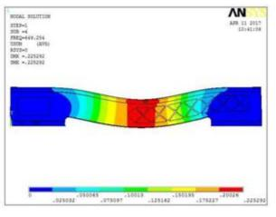
Fig 21: Natural Frequency mode - 4 Deformation
