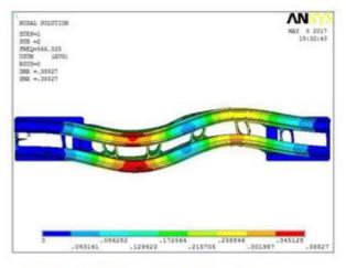
Fig 29: Natural Frequency mode - 2 Deformation
