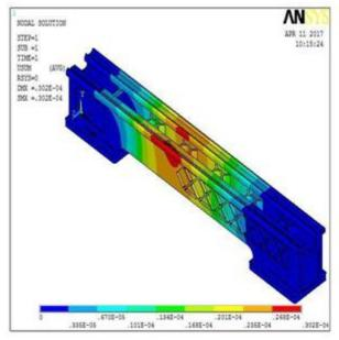
Fig 15: Deformation of lathe bed before weight optimization
