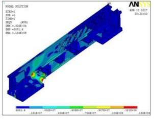
Fig 17: Von-mises stress Distribution of lathe bed before modification
