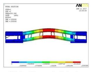
Fig 18: Natural Frequency mode - 1 Deformation
