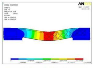
Fig 31: Natural Frequency mode - 4 Deformation
