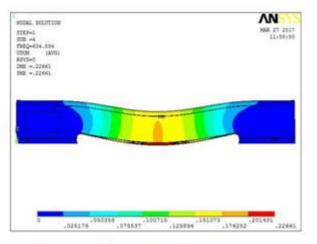
Fig 11: Natural Frequency mode - 4 Deformation
