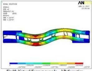
Fig 19: Natural Frequency mode - 2 Deformation
