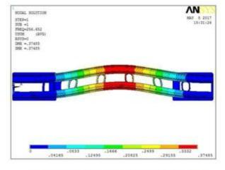
Fig 28: Natural Frequency mode - 1 Deformation
