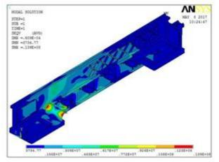
Fig 27: Von-mises stress Distribution of lathe bed before modification 286
