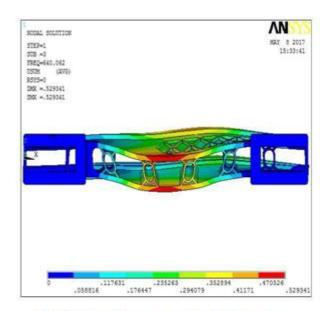
Fig 30: Natural Frequency mode - 3 Deformation
