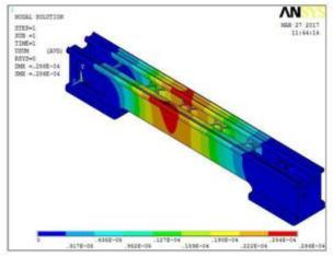
Fig 5: Deformation of lathe bed before weight Optimization
