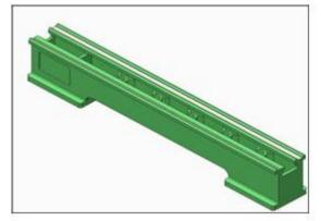
Fig 2: Solid model of lathe bed
