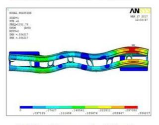
Fig 13: Natural Frequency mode - 6 Deformation
